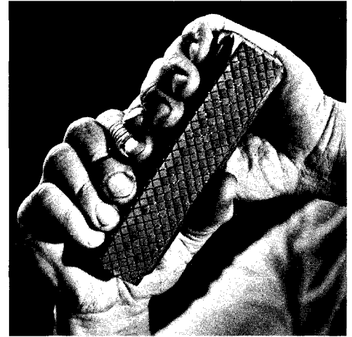
FIG. 103—Because the master laps will bend overall, small hand laps are also necessary.
