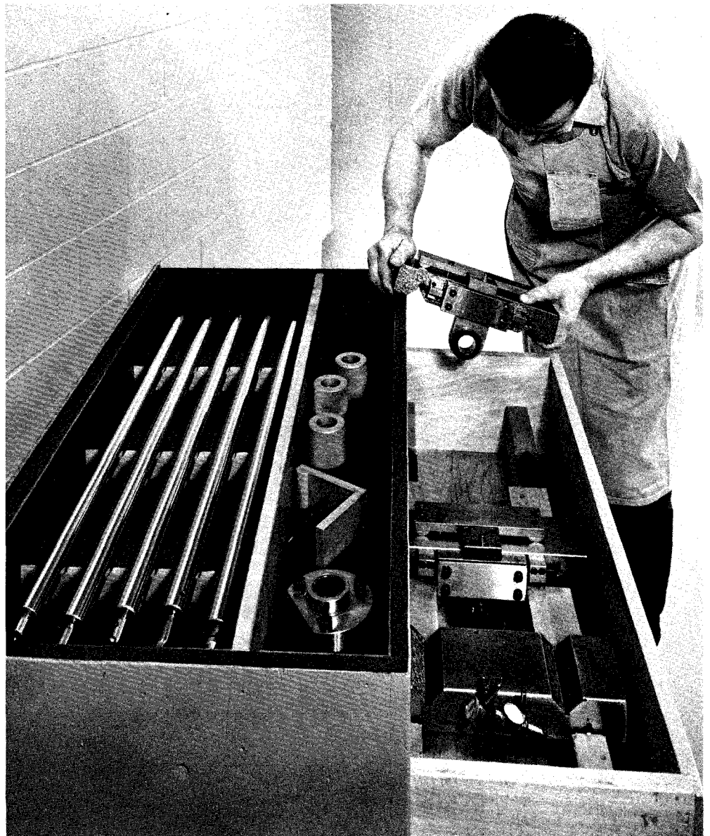
FIG. 301— Highly specialized equipment used to align the lead screw precisely in the base of the Measuring Machine.
