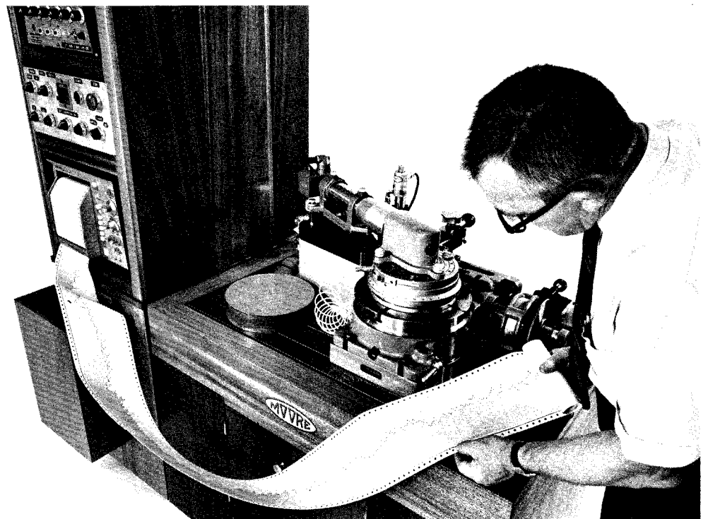
FIG. 385—The rotary table is calibrated and the error charted over one thousand, four hundred and forty positions in this automatic set-up. Time: 80 minutes. Note that worm-and-gear errors are clearly shown.
