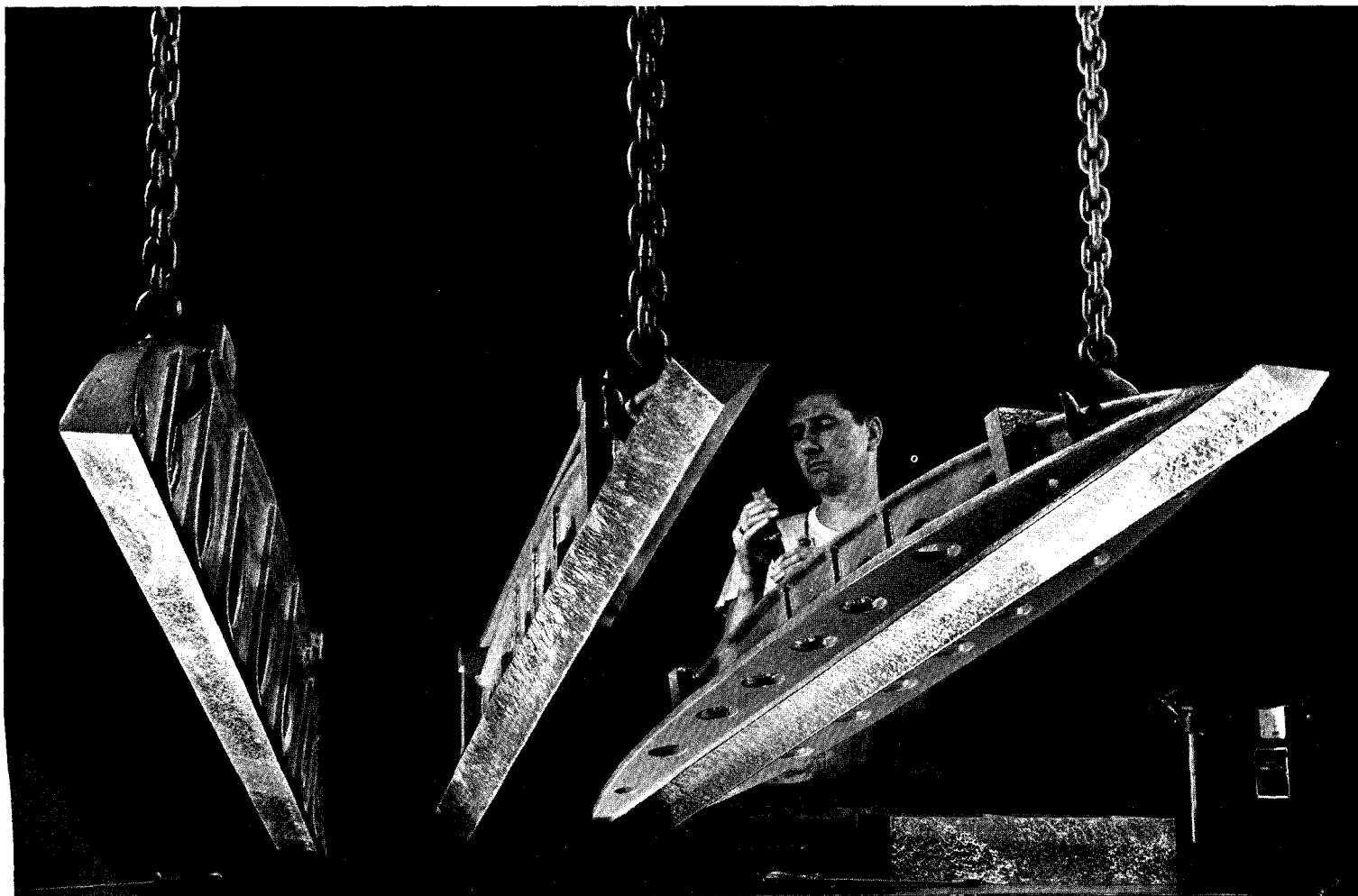
FIG. 28— The straightedges shown were at various times used as masters for machine ways, but were not self-proving, not sufficiently rigid, and unduly sensitive to temperature variations.
