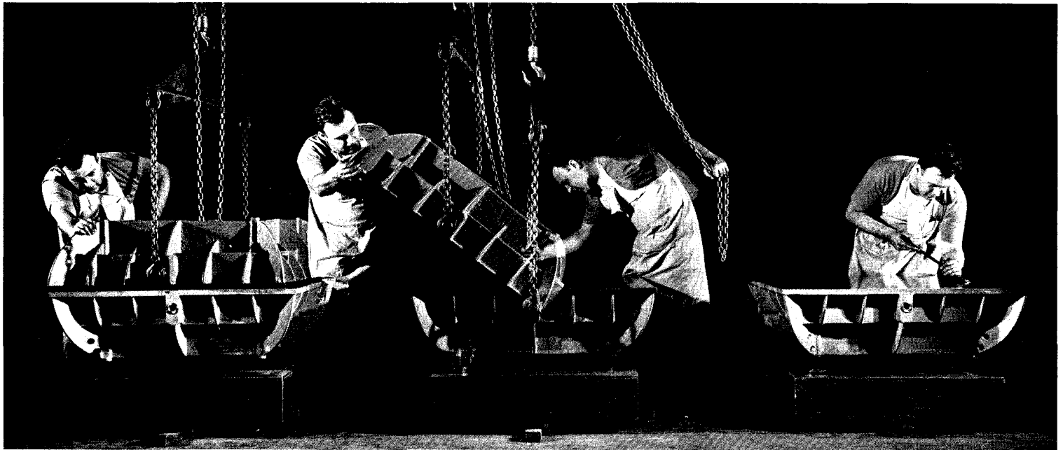
FIG. 7—By systematically matching three surface plates and scraping the high points of their contact, three flat planes are created, regardless of initial flatness of the plates.
