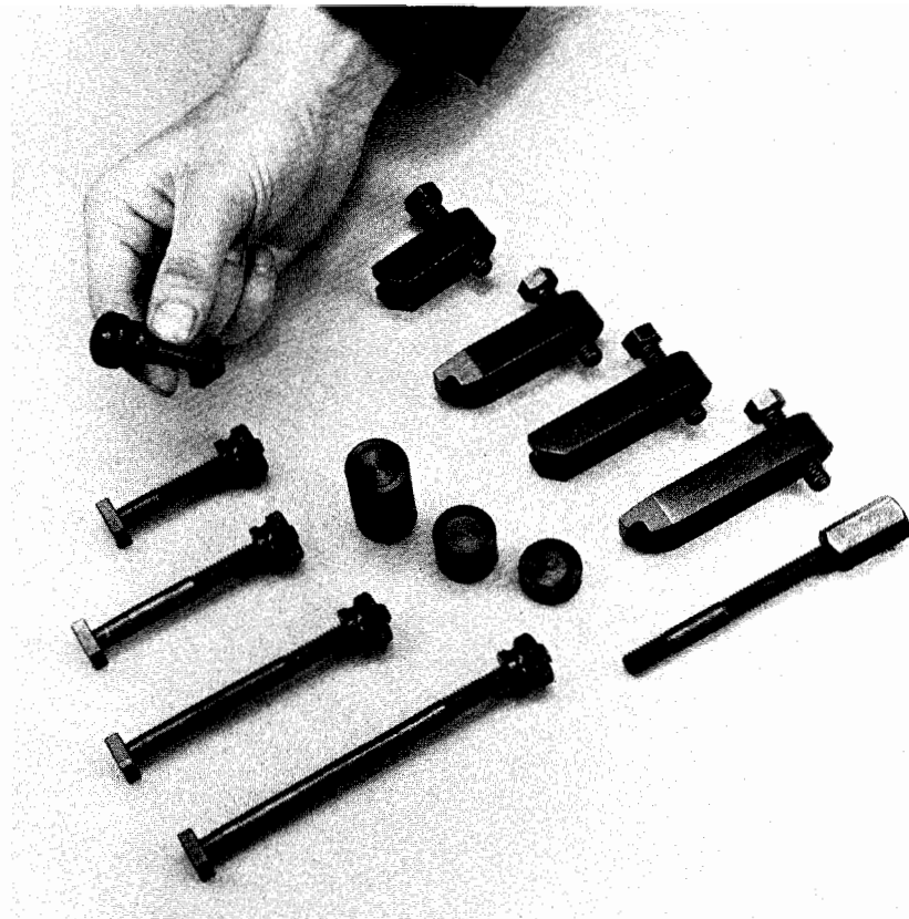
FIG. 473—A special set of workpiece clamps is furnished with the Universal Measuring Machine; a few such items are shown. An important feature of the set is the use of knurled nuts to avoid distortion of the workpiece through clamping-pressure.
