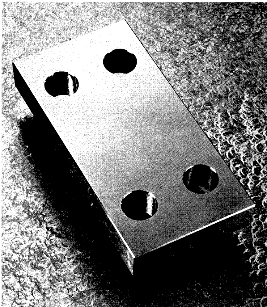
FIG. 474—This simple demonstration piece, measuring 4 inches by 8 inches overall [101.6 x 203.2 mm] and having four 1-inch [25.4 mm] holes, may be used to show most of the fundamental Universal Measuring Machine techniques.
