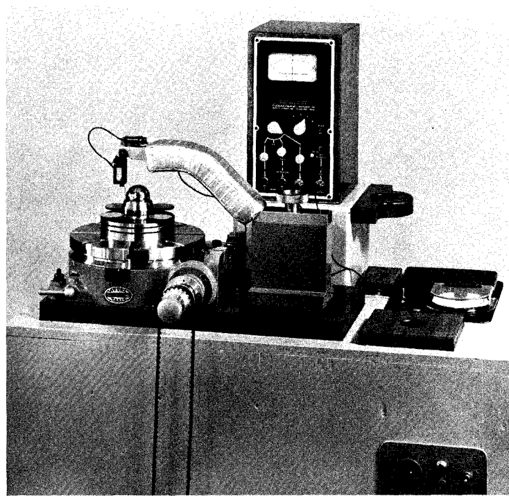
FIG. 364—A polar recording of rotary table "trueness of rotation" is made by reference to a master ball, round to .000001 inch [0.000025 mm]. The rotary table spindle is checked with axis vertical (shown), and while horizontal by using its built-in right angle feature.
