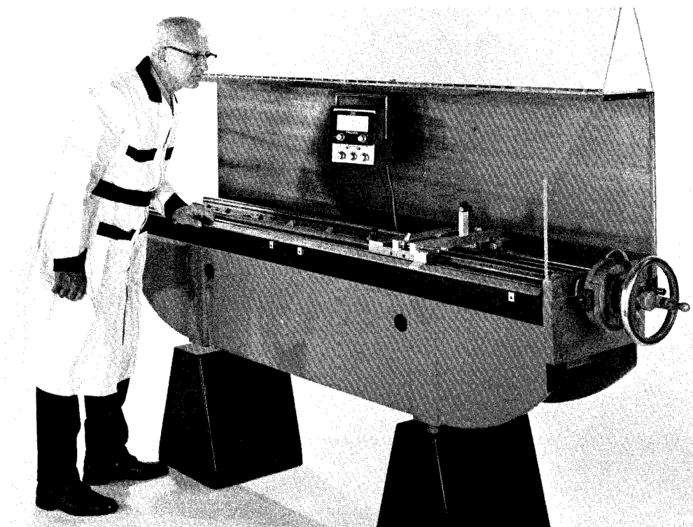
FIG. 546—The 72-inch Single Axis Measuring Machine has the capacity to measure lead screws, end standards, and line standards up to 72 inches in length [in metric 1830 mm]. A unique disengageable "nut" allows the carriage to be moved
