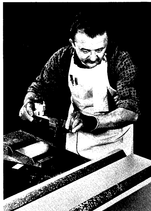
FIG. 46--Once the datum is set, the center-distance of the female double V master can be compared to the hardened master and scraped to agreement.
