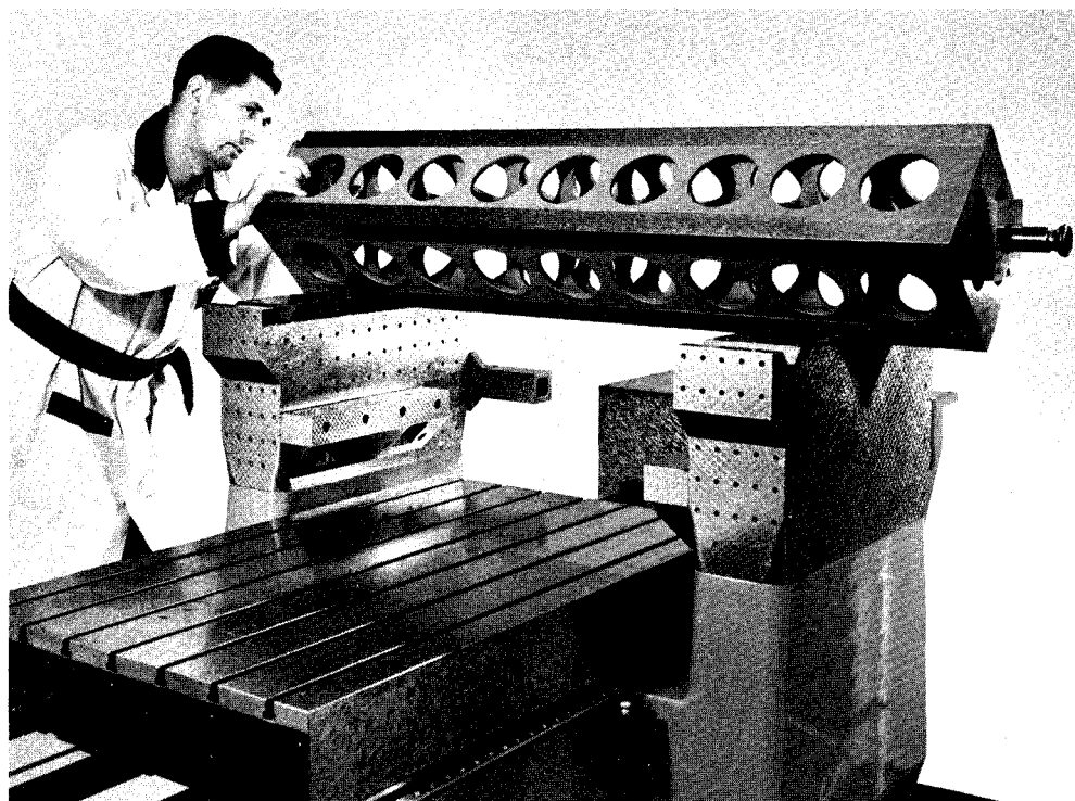
FIG. 554—The master box straightedge is used to establish the V-mounting surfaces for the two monorails of the M.I.T. "C" ruling engine.
