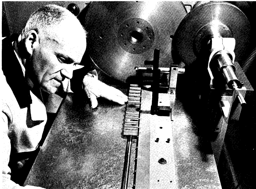
FIG. 285—Gaging faces of the Step Gage are lapped on a special fixture. Great care must be taken in the lapping operation to maintain the “geometry” of the faces. If
