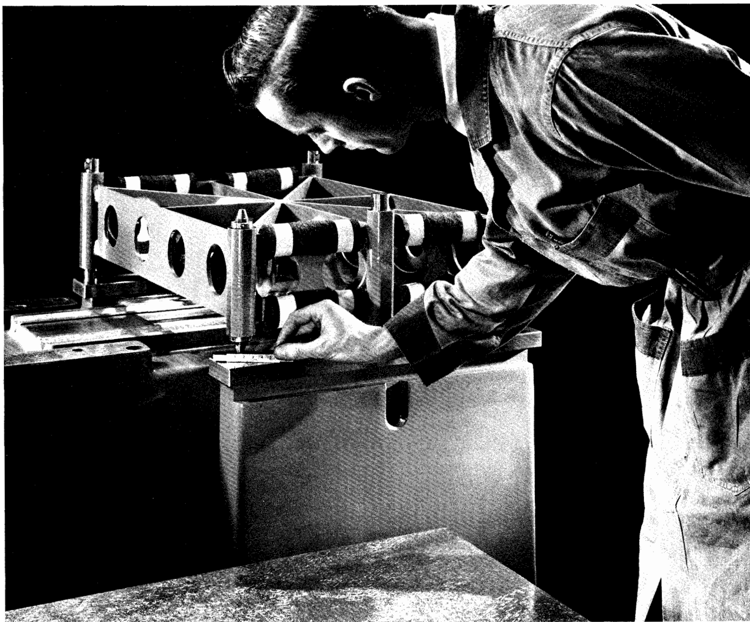
FIG. 116—One technique for measuring parallelism of the flat ways utilizes the three-footed twist gage—and simultaneously provides another working-check of straightness of each flat way. This method requires the use of a master surface plate as a datum and is self-checking.
