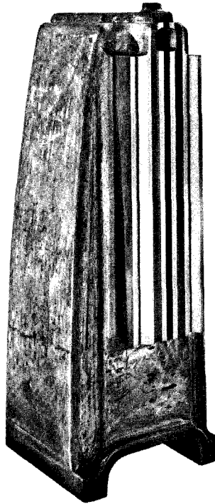
FIG. 95--No. 3 Measuring Machine column--rough-scraped.
