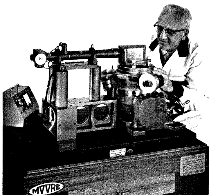
FIG. 401— The 1440 Small Angle Divider together with the standard granite plate in order to calibrate a precision rotary table.
