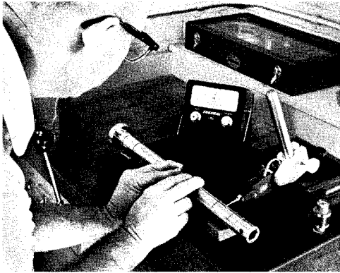
FIG. 438—Following a lapping operation, size and taper of the spindle shaft are inspected using an electronic indicator and stand.
