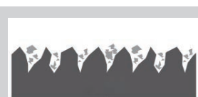
ORDINARY FILES Clogged with filing debris
