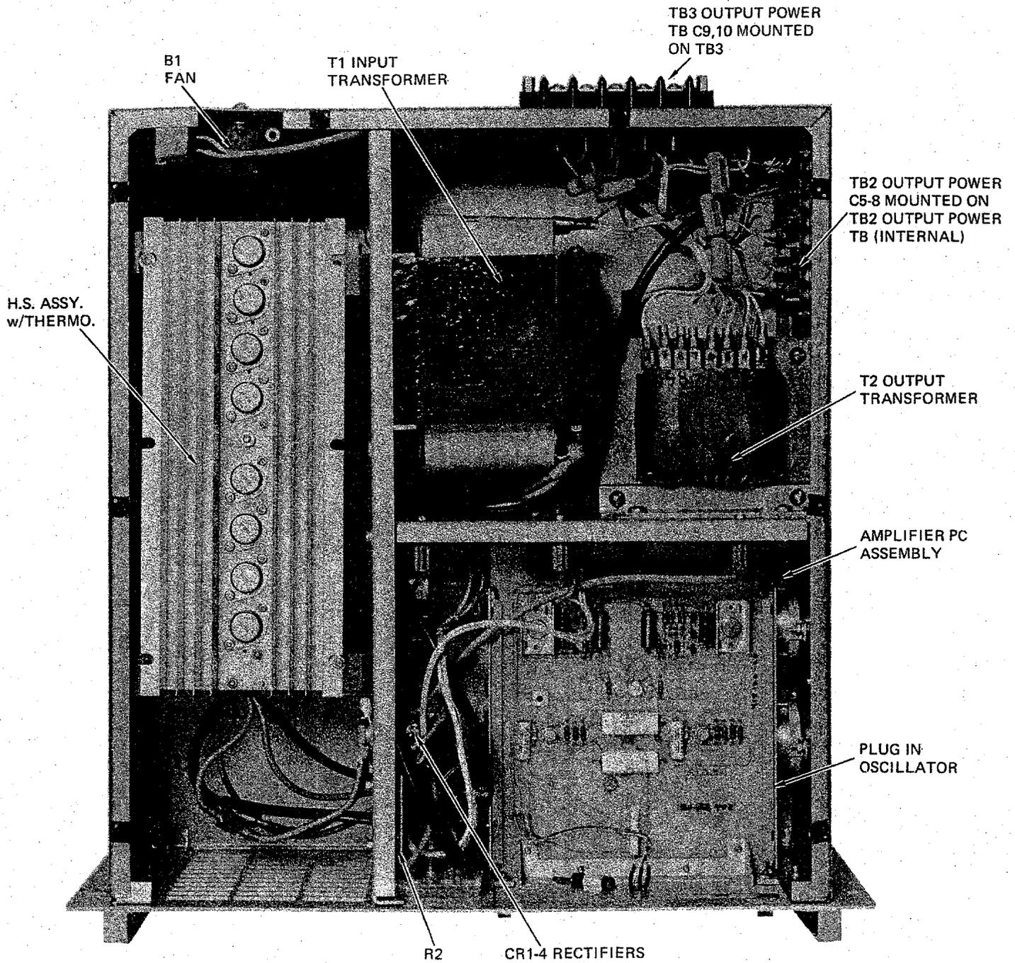
Figure 5-4. Model 501B Bottom View
