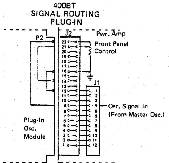
Figure 4-5. Signal Routing Plug-In Connections
