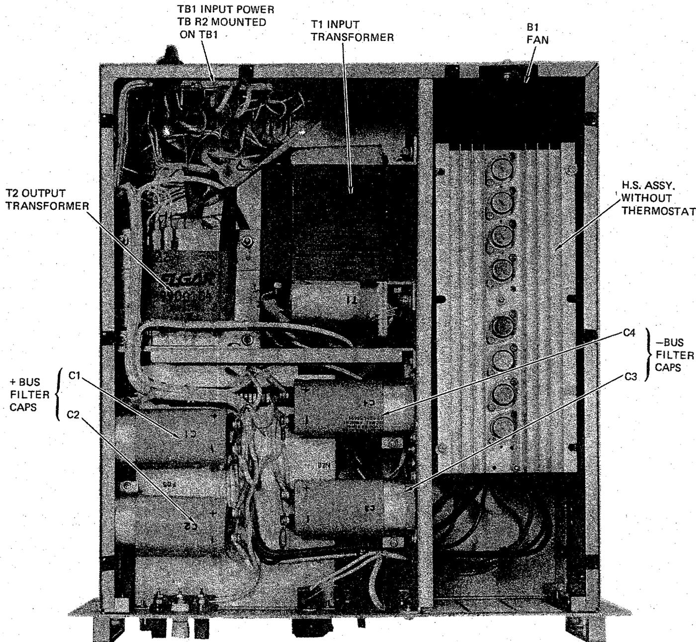
Figure 5-3. Model 501B Top View
