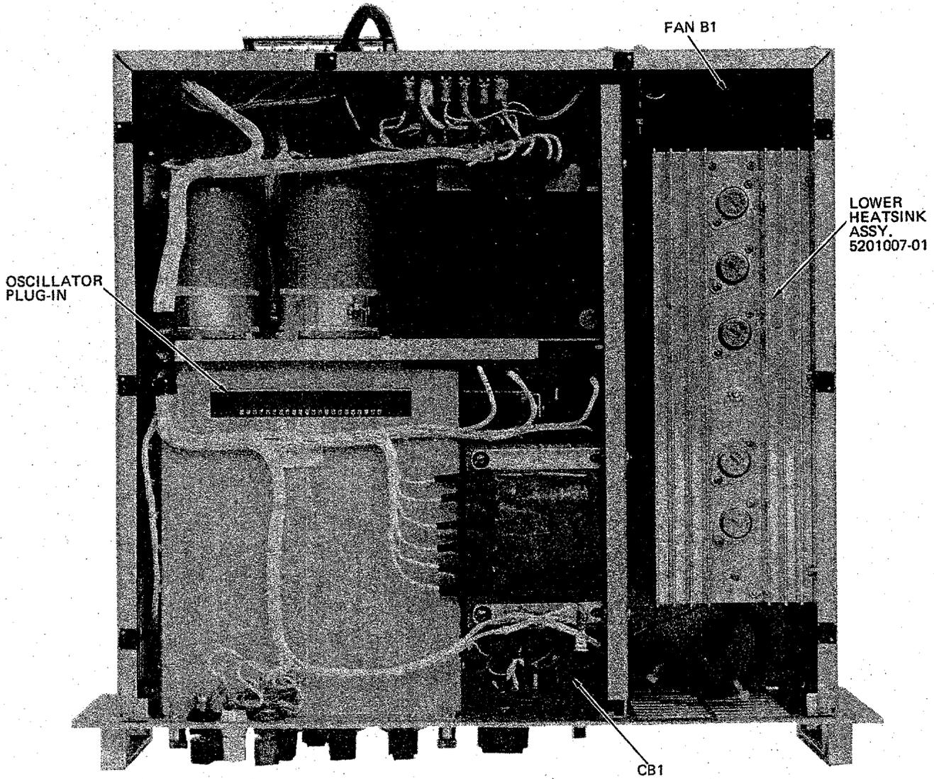
Figure 5-2. Model 251B Bottom View.
