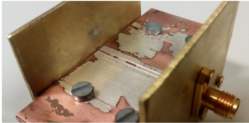
Figure 27 – CPWG lenght 30 mm with a 300 \mu m gap, using 2,92 mm SMK connectors.
