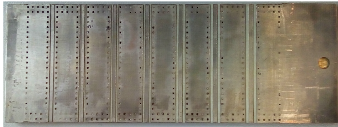
Figure 24 – Various CPWG with different gaps.
