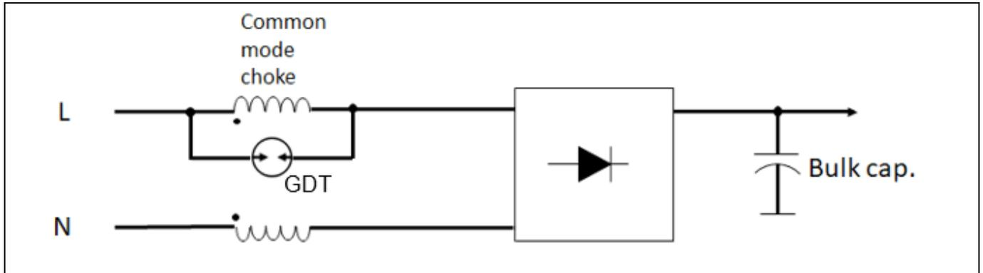
**Figure 15** GDT paralleled with CM choke for CM surge
