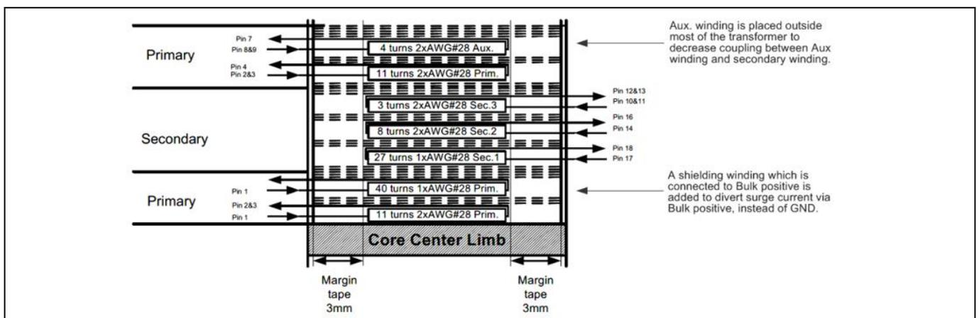
**Figure 18 Transformer winding design with shielding layer**
