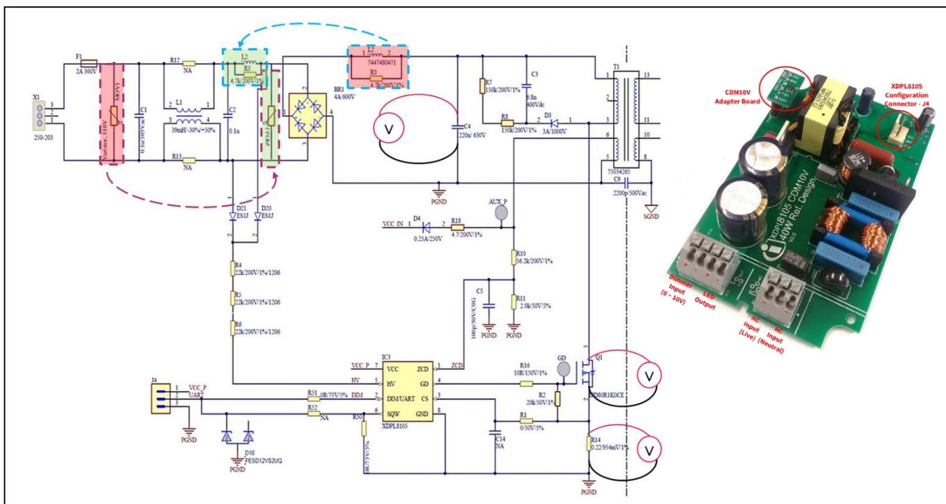
**Figure 20** Line filter – original and rearranged design for the [REF-XDPL8105-CDM10V \[3\]](#)
