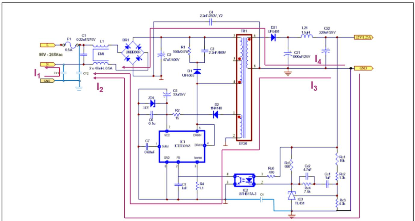
**Figure 16** Example of SMPS for surge test
