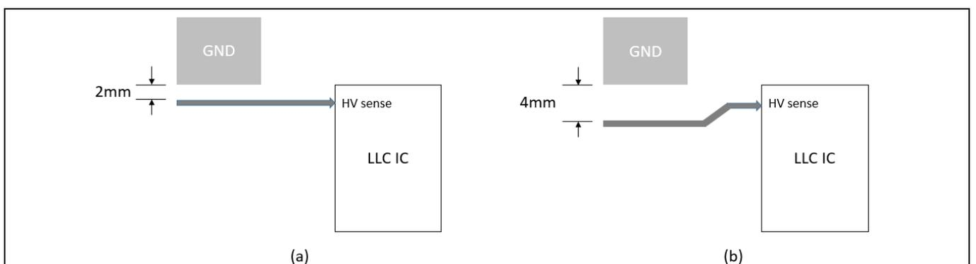
**Figure 27** Original layout (a), changed layout (b)
