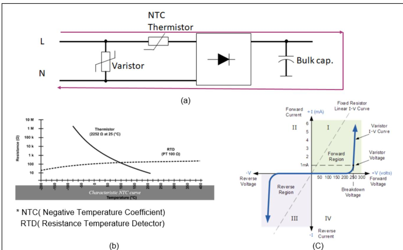
Figure 12 DM surge (a), Characteristic curve of NTC (b), Characteristic curve of varistor (c)
