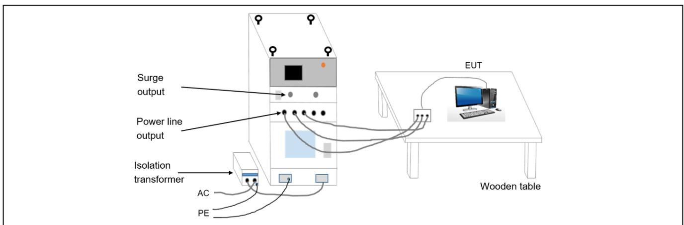
**Figure 5** Test setup
