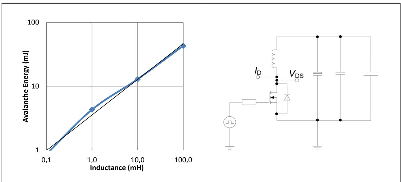
Figure 11 Avalanche energy vs. test inductance, data for IPx80R900P7 [2]
