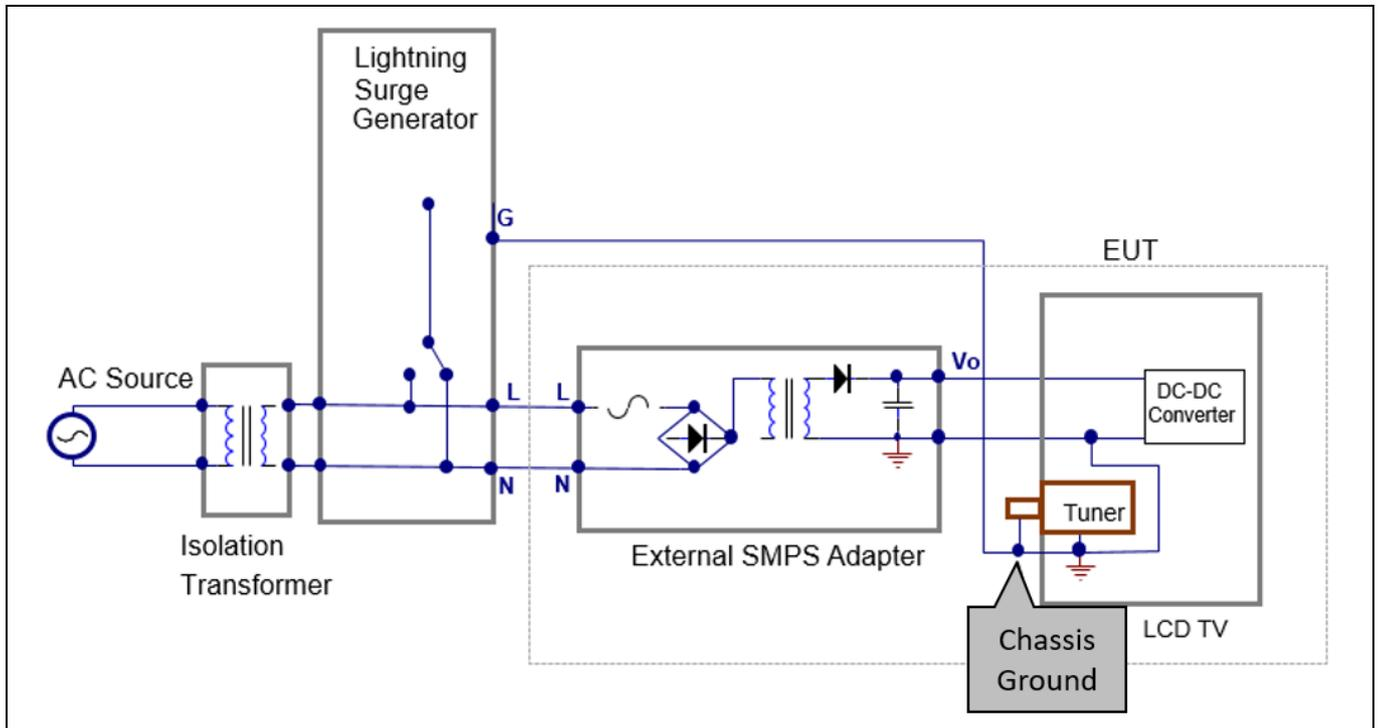
**Figure 6** Example of LCD TV Power test setup
