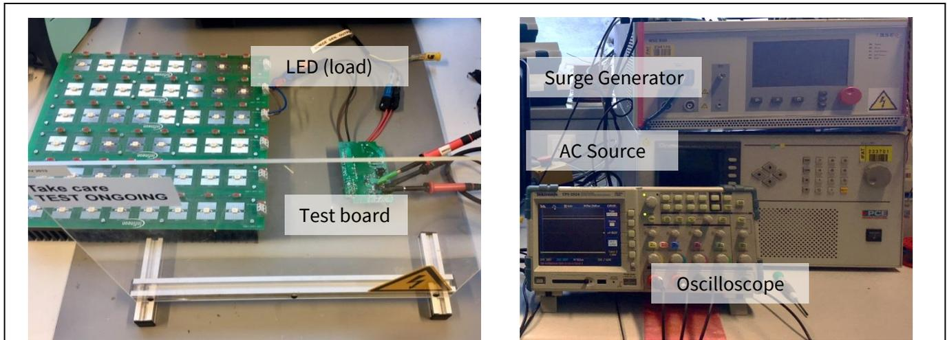
**Figure 23** Line-to-line measurement setup
