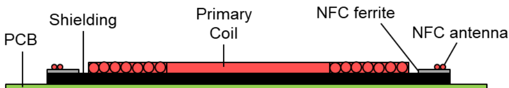
Figure 58. Example of NFC antenna outside the Primary Coil
