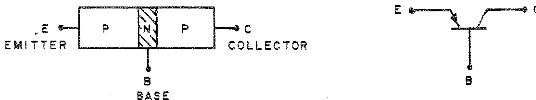
Figure 4-1. PNP Transistor and Circuit Symbol
